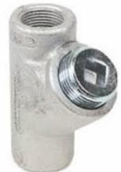
Seal-offs prevent explosions from spreading through conduit systems and igniting outside atmospheres. When properly installed and filled with a UL-listed sealing compound, they create a physical barrier that minimizes passage of explosions from traveling freely through the conduit.
